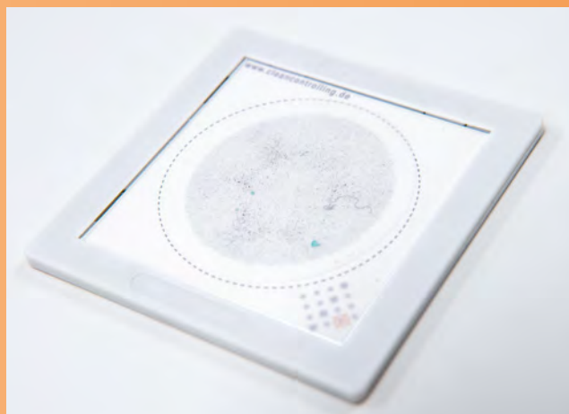
Framed particle filter from the clean room with separated particles
