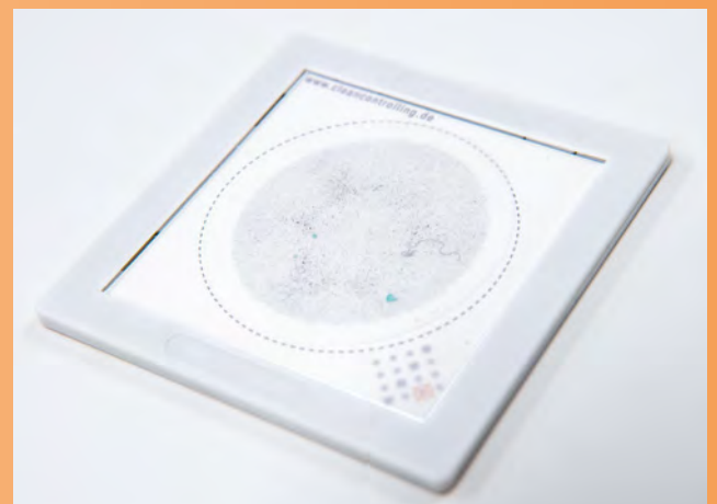
Framed particle filter from the clean room with separated particles
