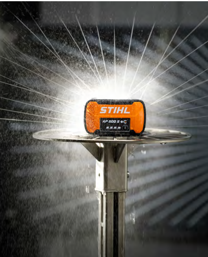
The rain test demonstrates the robustness of the battery pack when used in wet weather.
